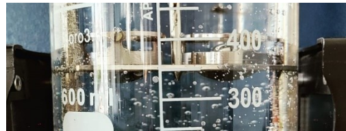
Bitumen softening during a Ring and Ball Test.
