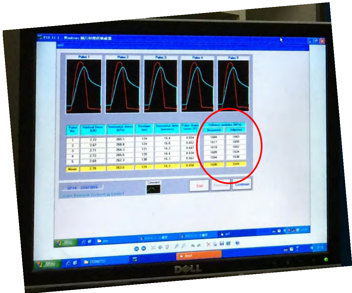
Figure 7: Screenshot of typical ITST results. In red values of stiffness modulus measured.
