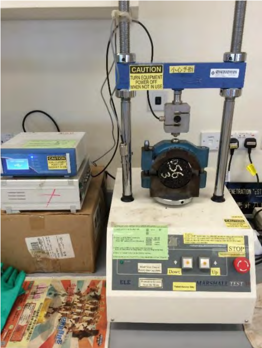
Figure 4: Machine used for Marshall test (in the middle a sample can be seen)
