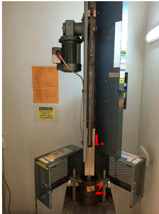
Figure 3: Compaction equipment. Legend : 1. Hammer 2. Moulded sample
