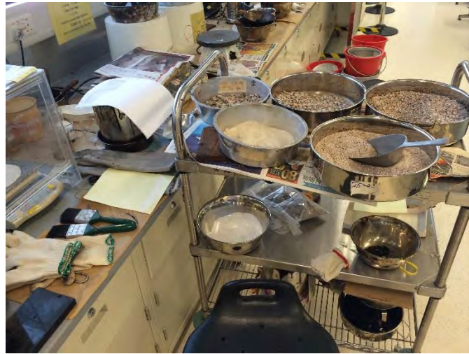
Figure 1: Containers with separated aggregate sizes before weighing (from 10mm diameter to fillers (<75 microns))
