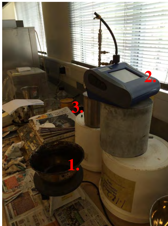
Figure 2: Picture taken by preparing the mixture. Legend : 1. Mixture 2. Equipment measuring PM 2.5 content 3. VOC canister collecting air sample
