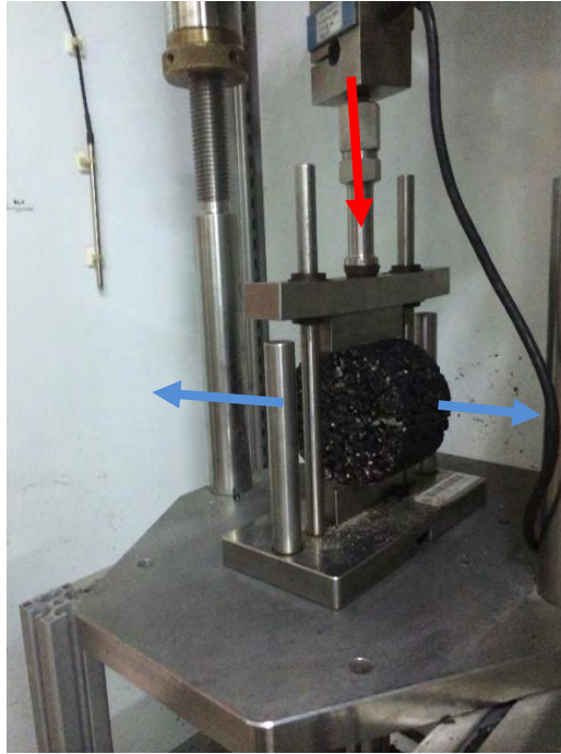
Figure 8: Sample installed in the fridge (test at 20°C) for Fatigue resistance test. Red arrow stands for load direction and blue arrows for direction of main deformation. Main crack will appear in parallel with load direction
