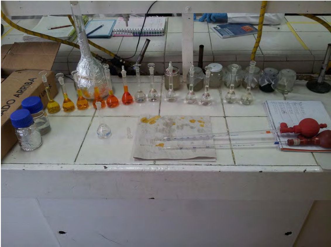
Figure 33: Experimental setup for the nitrite analyses of the samples (the increasing intensity of the reddish tone on the 6 tubes on the left indicate increasing concentrations of nitrite used to construct the calibration curve)
